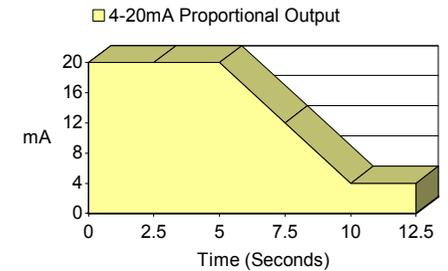
**Fig. 6** Typical Response after last Flame seen - IR<sup>3</sup> Flame Sensor
