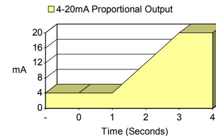
**Fig. 5** Typical Response on seeing Flame - IR<sup>3</sup> Flame Sensor
