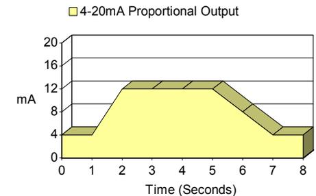
**Fig. 7** Typical Response to Burst of Flame - IR<sup>3</sup> Flame Sensor
