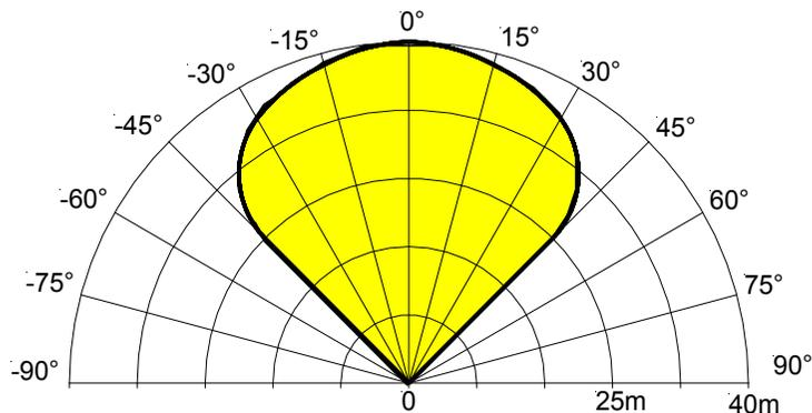
**Fig. 3** Relative range as a function of viewing angle - IR<sup>3</sup> Flame Sensor
