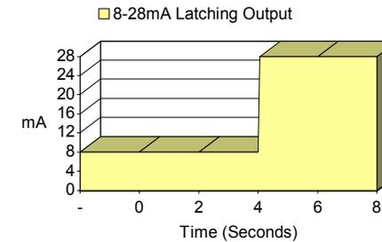
**Fig. 4** Typical Response on seeing Flame - IR<sup>3</sup> Flame Sensor
