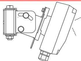
Fig. 9 Adjustable Mounting Part number: 007127
