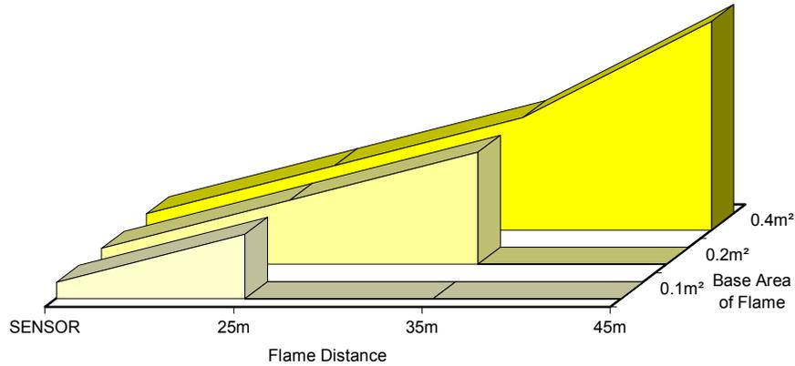
**Fig. 2** Sensor centre line detection range for n-heptane fire (yellow sooty flame) - IR<sup>3</sup> Flame Sensor, sensitivity set high for class 1 performance
